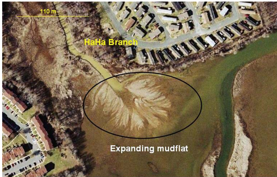
Figure 2.4.6 Aerial image of HaHa Branch showing a sediment plume been delivered into the OPC estuary.
