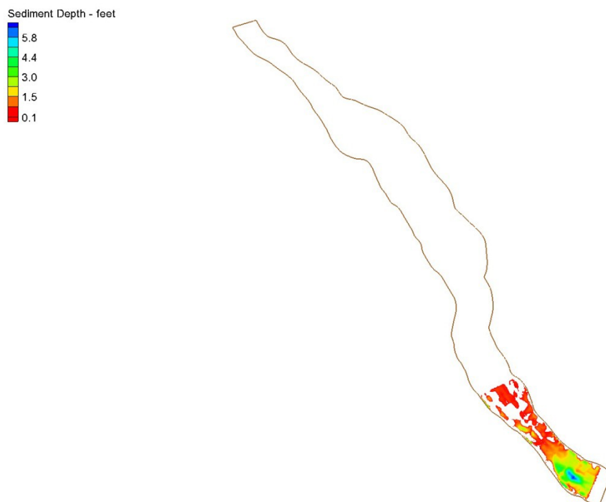
Figure 29 Additional sediment depth added to the 2011 bathymetry for the full reservoir simulation
