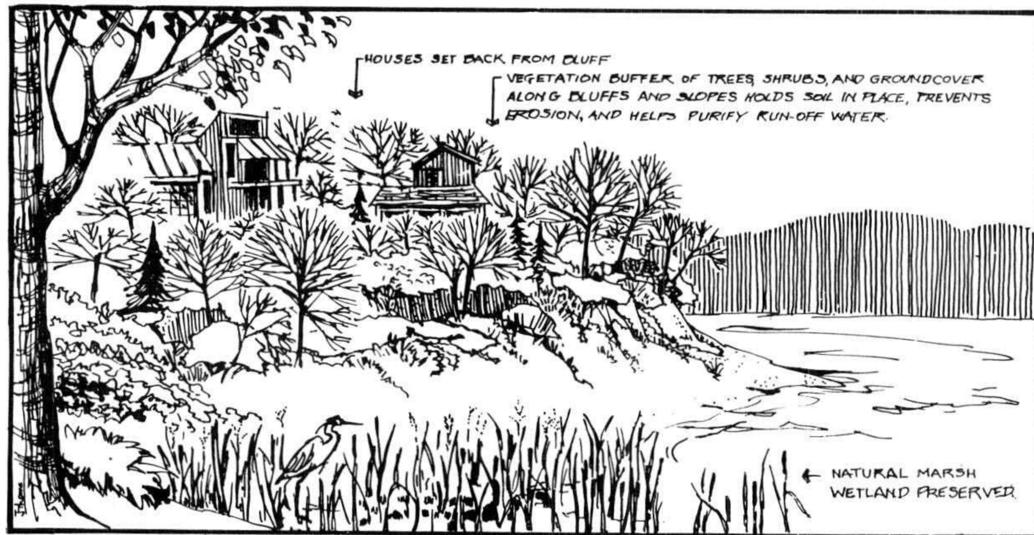
Sketch showing use of vegetation as buffers near an urban wetland area.
