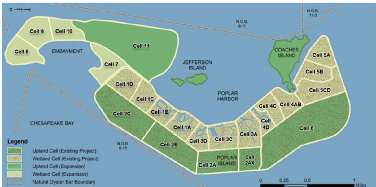
Figure 1B: Paul S. Sarbanes Ecosystem Restoration Project at Poplar Island - Site Layout and Cell Designations
