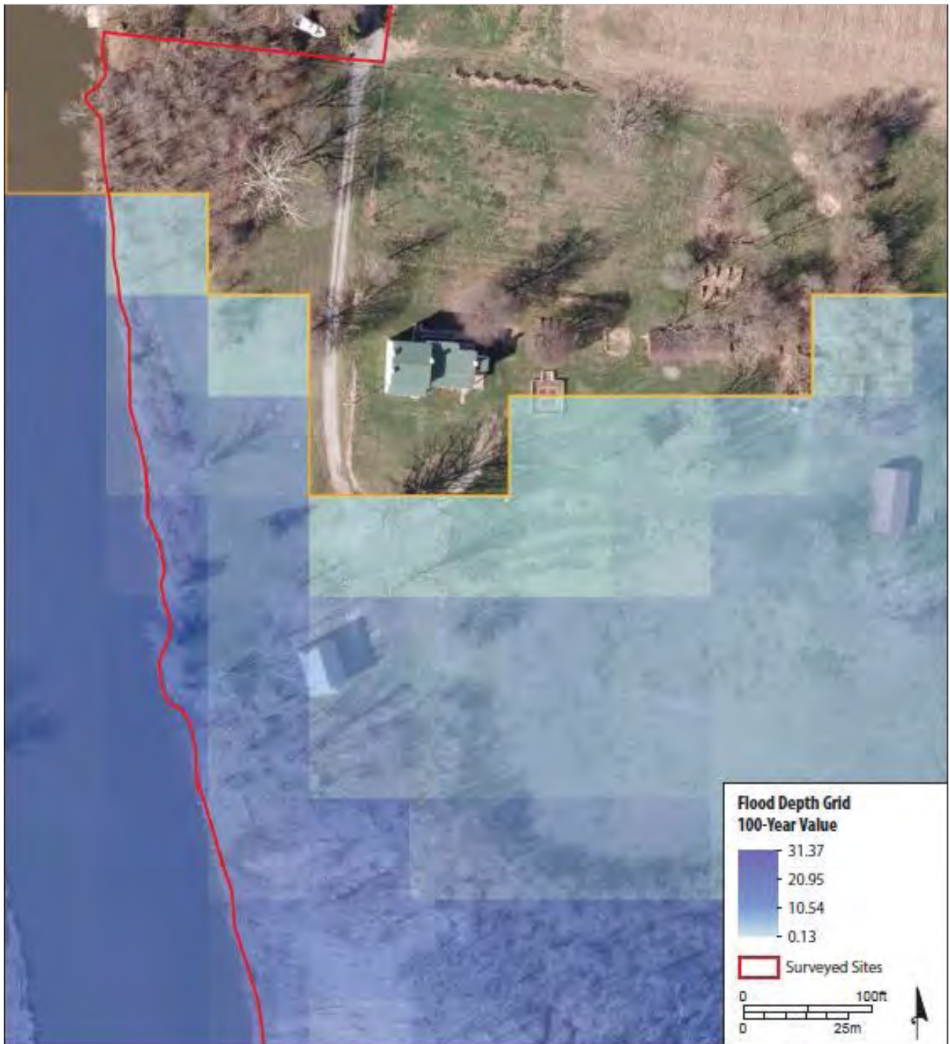
Figure 2.18 - The map generated using the Hazus-MH Riverine flood model indicates this historic house, located on the Eastern Shore, is located outside of the 100-year floodplain, or Special Flood Hazard Area (SFHA).
