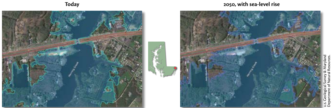
Figure 17. Areas of Ocean Pines that would be flooded by 1.5 m (4.9 ft) storm surge from a Category 2 hurricane today (left) and in 2050 after sea-level rise of 15 cm (0.5 ft), which is the current rate of sea-level rise (right). 10 However, the rate of sea-level rise is projected to increase above the current rate in the future, so this map likely underestimates the extent of flooding in 2050.
