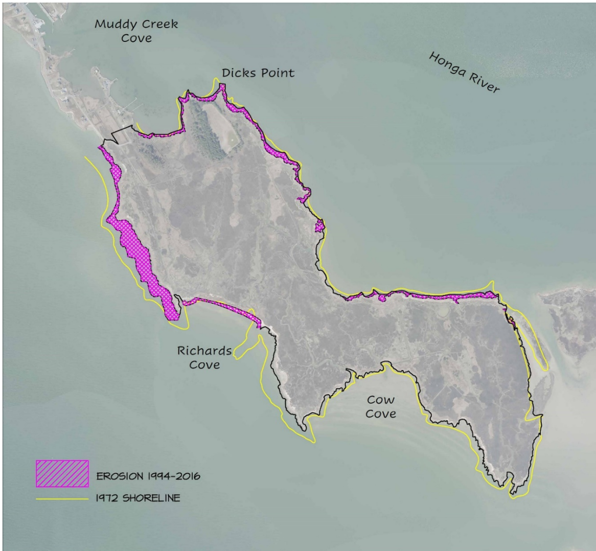
Figure 19 - Erosion along the South Marsh Shoreline
