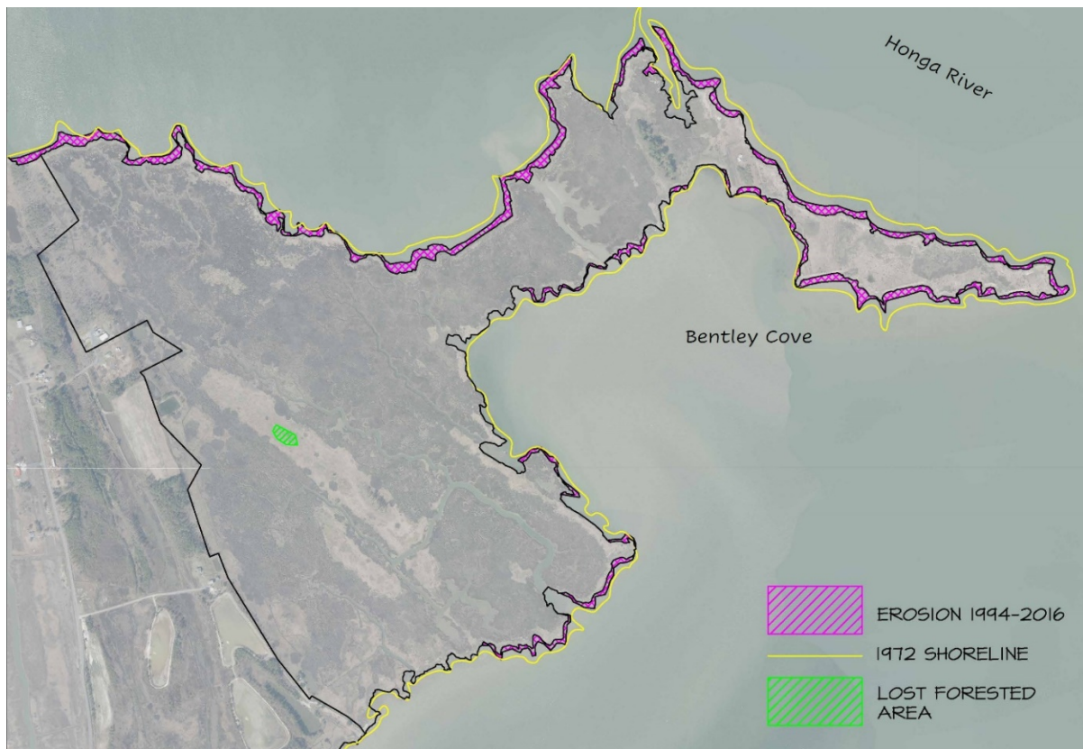
Figure 11 - Erosion and Lost Habitat along the Northeast Marsh Area
