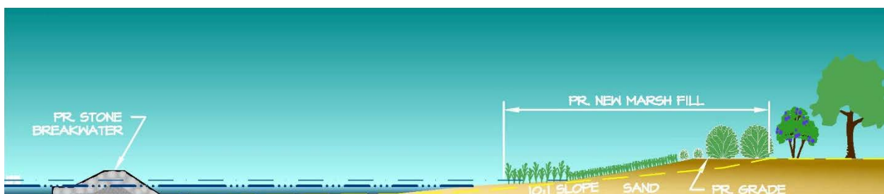
Figure 48 - Stone Breakwaters and Marsh against Coastal Erosion
