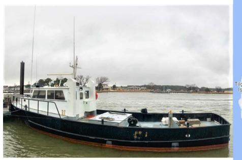
M/V H.J. ELSER / Service Area BUILT: PAASCH Marine Services YEAR: 1967 LENGTH: 50' WIDTH: 14.5' DRAFT: 6' TON: 32 PROPULSION: 600 HP TWIN SCREW DIESEL
