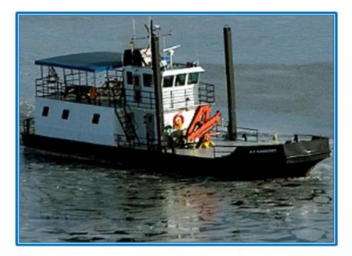
M/V A. V. SANDUSKY / Service Area BUILT: GENERAL SHIP REPAIR (1989) LENGTH: 80' WIDTH: 24' DRAFT: 4.5' 120 TON ICE BREAKING CAPABILITIES: 8" PROPULSION: 700 HP TWIN SCREW DIESEL ENGINE
